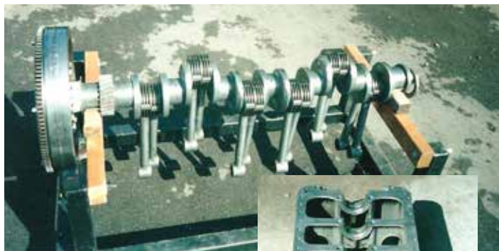
Above: J12 Crankcase with finned and pinned rod caps
