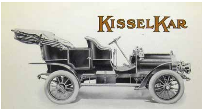
The 1907 KisselKar Model "C." For $1850 f.o.b. Hartford, you could acquire this 30 H.P., four-cylinder (cast in pairs, 4-1/2" x 4-3/4" bore x stroke), 98" W.B., three-speed, open drive shaft, 2250 lb, 5-passenger motor car with internal and external rear brakes. McDuffee Auto Company, Chicago and Milwaukee, was the sole sales agent. (From a 1907 Kissel sales brochure)
