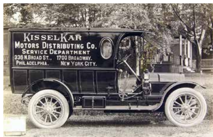
The 1910 KisselKar Delivery Wagon. Kissel first trucks appeared in 1908 with specialized bodies on a car chassis. In 1910 Kissel introduced its first trucks on specialized chassis. By 1912 the Kissel truck line extended up to a 5-ton, 156" chassis. (Wisconsin Automotive Museum.)
